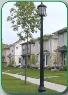
Non cut-off fixtures contribute to light pollution.
